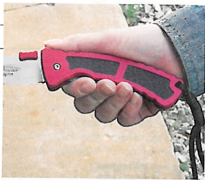
The author recommends softening the sharp edges on the grooves in the underside of the aluminum handle.
